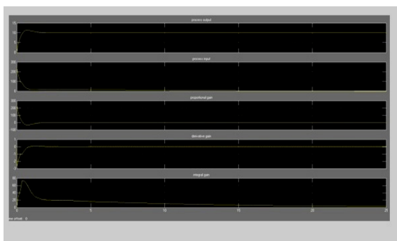
Fig 8: Output response for total head using Fuzzy tuned PID controller
